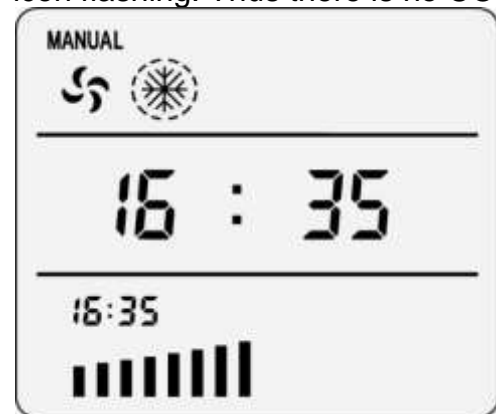
Picture 4-2 pump stop running (water shortage)
